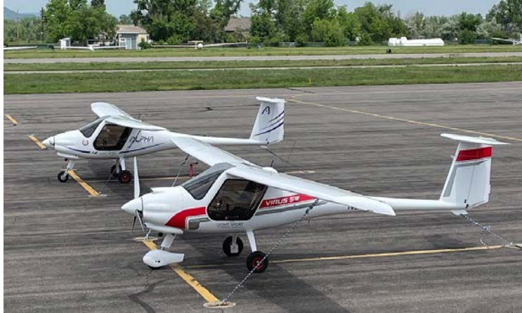
Figure 8: With a take-off noise rating of only 71db 3 , Journeys' two Pipistrel airplanes are several times quieter than typical training aircraft such as Cessna 172s which have a take-off noise rating of 78-85 db 4 or Cessna 182s, which have a take-off noise rating of 81-88 db 5 .
