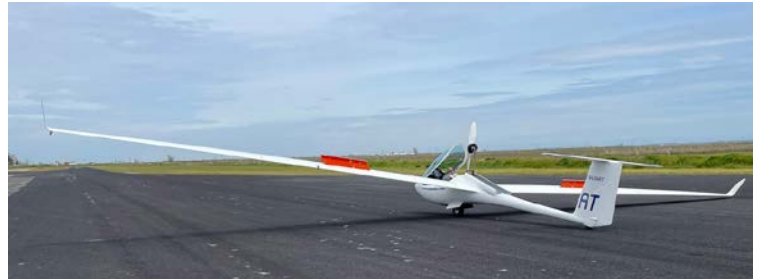
Figure 6: This electric self-launching AS 34Me, serial number 5, one of the first in the world, began operating at the Boulder airport in 2023. It has a quiet electric motor, operates emissions-free, and can take off without assistance by a tow plane. The picture shows the glider prior to its inaugural flight at Williams, CA.
